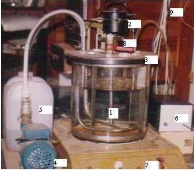
Figure 1. Functional Bioreactor. 1. Glass vessel; 2. DC motor; 3. Stainless top plate; 4. Water pump; 5. Cooling tank; 6. Power unit; 7. Basement; 8. Gear system; 9. Wires to control computer.
